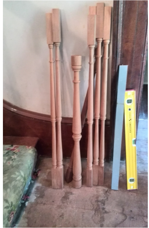
The newly turned balusters and newel post, awaiting installation
